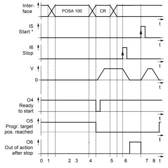
When using this START, a processing command interrupted by STOP and specified by a interface is restarted.
